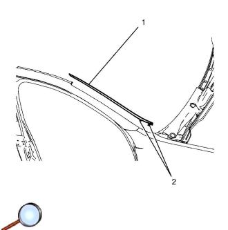
**Important:** Align the locating marks on the reveal moulding (2) with the locating marks on the windshield .
