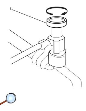
Note: Turn the HP and LP shut off valve taps (1) clockwise.
