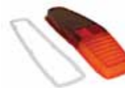
LENS & GASKET TAIL LAMP HQ, HJ, HX, HZ : WAGON, UTE & VAN PART NO. LRS1017
