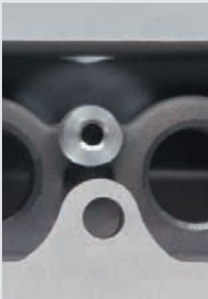
Lifter Boss Detail A
